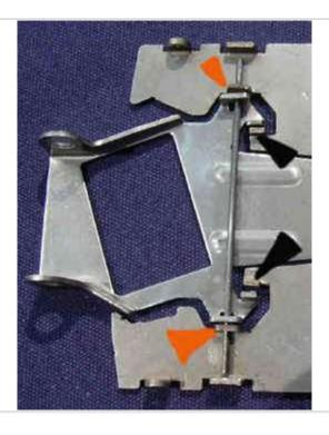
E2.3.8 JK X32 chassis for Super Production: The 64mm width regulation applies in these classes. Due to the manufacturing techniques, chassis may be delivered with the pan spread slightly at the rear so as to exceed the 64mm limit. The following methods only, are permitted to rectify this:
